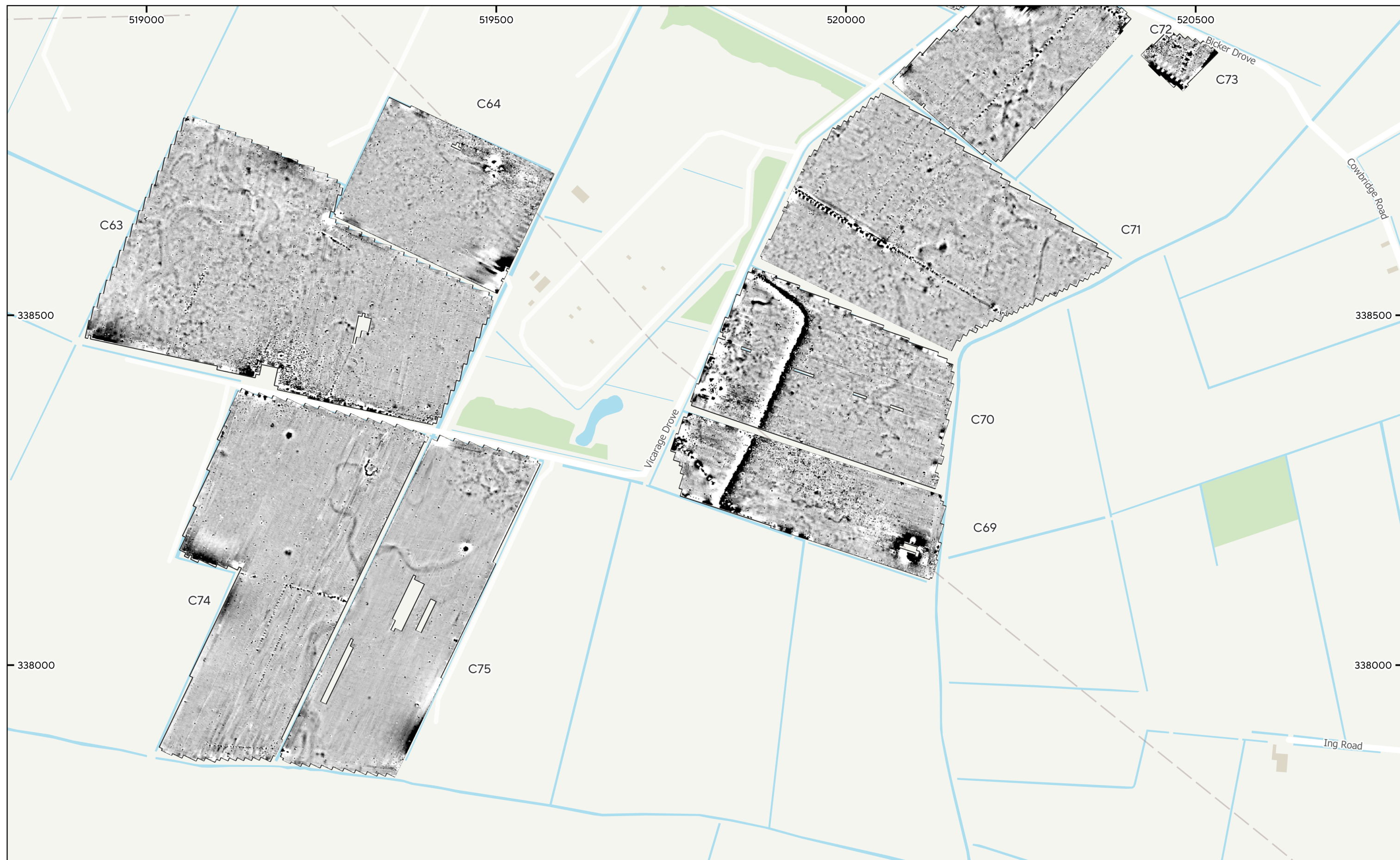
MSTF1735 - Beacon Fen Cable Route, Lincolnshire Figure 26 - Magnetic Total Field (Lower Sensor) (Cable Route Areas C63-C64 & C74-C75) 1:5,000 @ A3 © Magnitude Surveys 2024 Contains Ordnance Survey data © Crown Copyright and database right 2024
